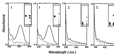
Fig. 2. Results of TLC and UV spectra of 2,4-pentanedione (—) and after oxidative reaction (---;21h) by PAn/ $\text{O}_2$  system (1),  $\text{KO}_2$ /THF (2),  $\text{H}_2\text{O}_2$ /FeCl<sub>2</sub> (3),  $\text{H}_2\text{O}_2$  (4).
