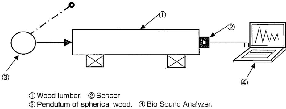
Fig.2 Experimental system using pendulum of spherical wood and a tapping sound analyzer.
