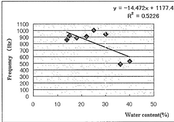
Fig.8 Changes in the frequency component of Japanese cypress with different water contents.
