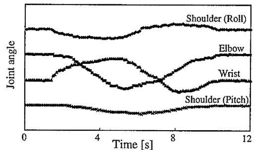
Fig.10. Joint-angle trajectory of robot arm tracing a circle
