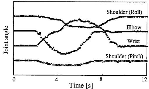
Fig.8. Joint-angle trajectory of robot arm tracing rectangle
