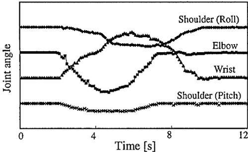
Fig.12. Joint-angle trajectory of robot arm tracing an inclined line
