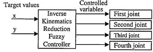
Fig.2. Block diagram of the Fuzzy Controller
