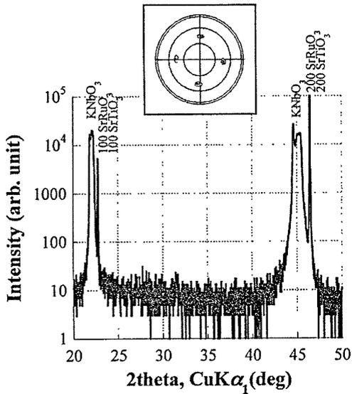
Fig.1 XRD pattern of KNbO<sub>3</sub> film deposited on (100)<sub>c</sub>SrRuO<sub>3</sub>//SrTiO<sub>3</sub> substrate together with the X-ray pole figure measurement fixed at 2θ of 31.5°.
