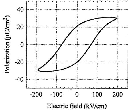
Fig.4  $P-E$  hysteresis loops measured at 100 kHz and maximum applied electric field of 196 kV/cm.
