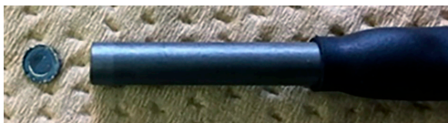
Fig. 3 Photograph of conventional tough hydrophone front plate and main body
