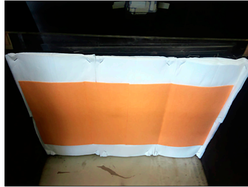
図 3. Water absorptive paper and polymer attached to inner tank wall.)
